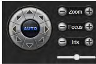
**PTZ Control:** You can use eight directional keys to rotate front-end devices, and AUTO indicates auto-rotation.
